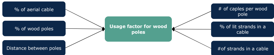
Exhibit 4.12: Algorithm for calculating the usage factors of the wood poles for the dark fibre service [Source: Axon Consulting]
